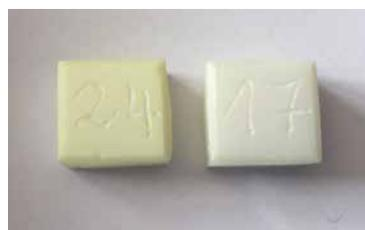
**Fig. 9:** Sample 24 was sintered on a closed Saggars (muffle). Sample 17 was inside the Saggars in the same firing run in a contaminated furnace.
